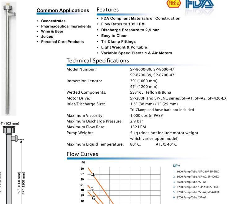
Note: Pump is constructed with FDA compliant materials; however, the system does not have FDA certification. \*Pump is intended for intermittent use.
